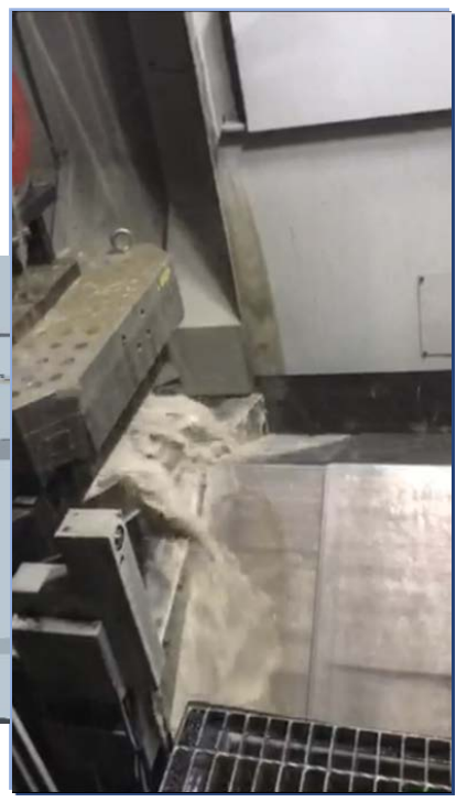
Chips on the upper surface of the rotating body of the table
